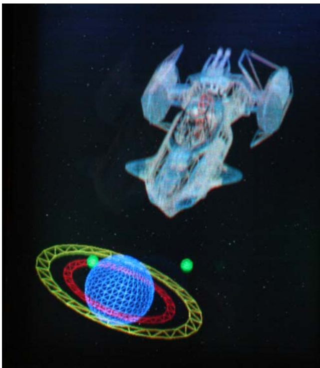
Fig. 7. 2D photo of color hologram on current prototype (camera focusing on planets)
